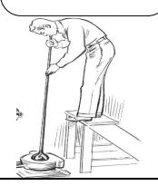
The gatherer shapes the hot glass by rolling it on a "marver" or machined iron plate.
